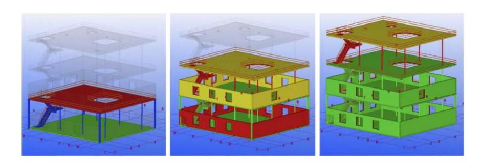
4D simulation (orange required safety equipment; green is completed; blue in progress; red in 1 week; yellow in 2 weeks).
