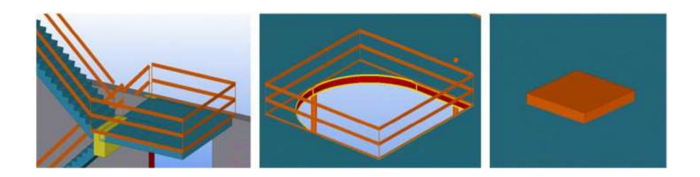
Examples of protective equipment for staircases, slab edges, and slab openings with different shapes/dimensions.
